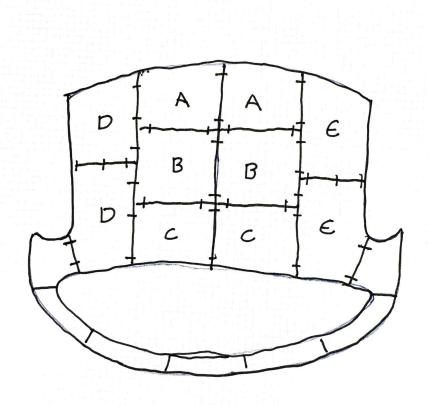
Once all panels are joined in pairs, attach A, B,& C. When the 6 middle panels are connected you will be able to mount the D & E panels to the ABC panels.
